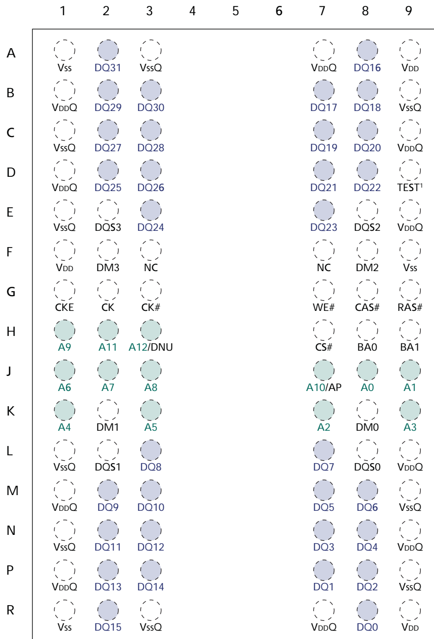
Figure 5: 90-Ball VFBGA Ball Assignments – 8mm x 13mm (Top View)
