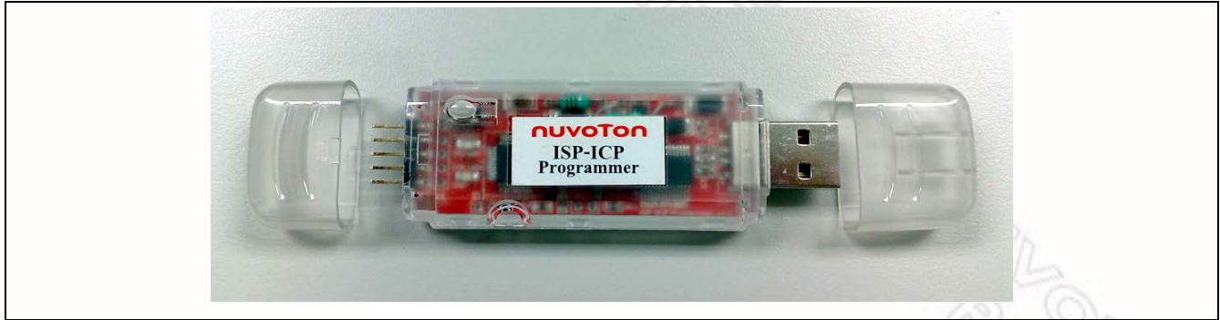
Figure 27–2 Nuvoton ISP-ICP Programmer
