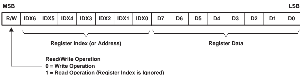
Figure 24. Control Data Word Format for MDI
