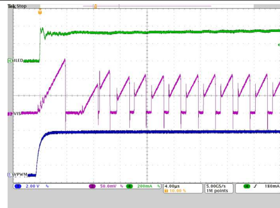
Ch1: External PWM input voltage; Ch3: Switch sense current resistor voltage; Ch4: LED current; Time: 4 μs/div
