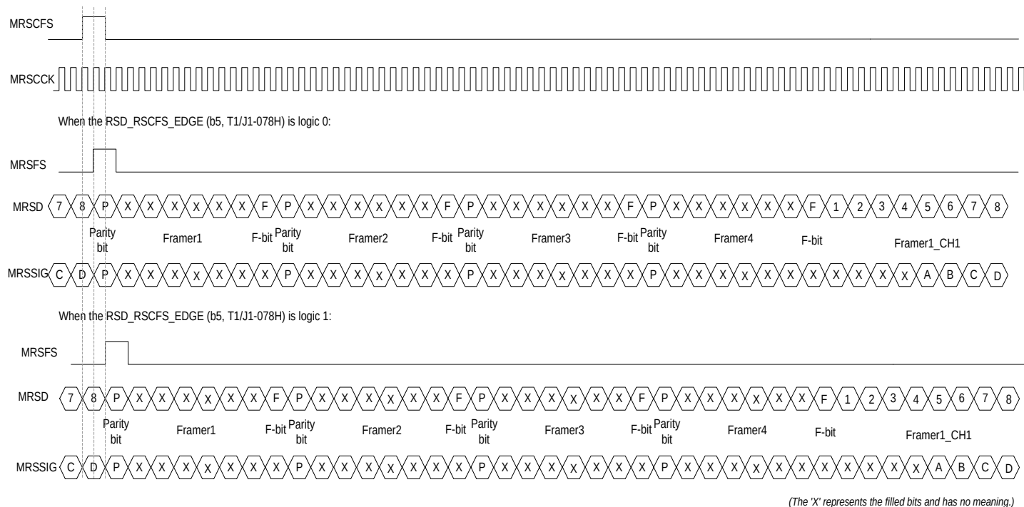
Figure 34. T1/J1 Receive Multiplexed Mode - Functional Timing Example 2
