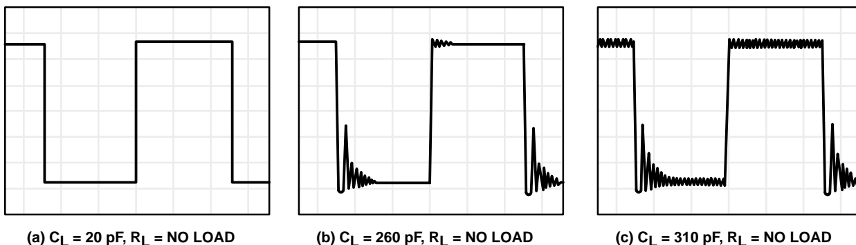
Figure 112. Effect of Capacitive Loads in Low-Bias Mode
