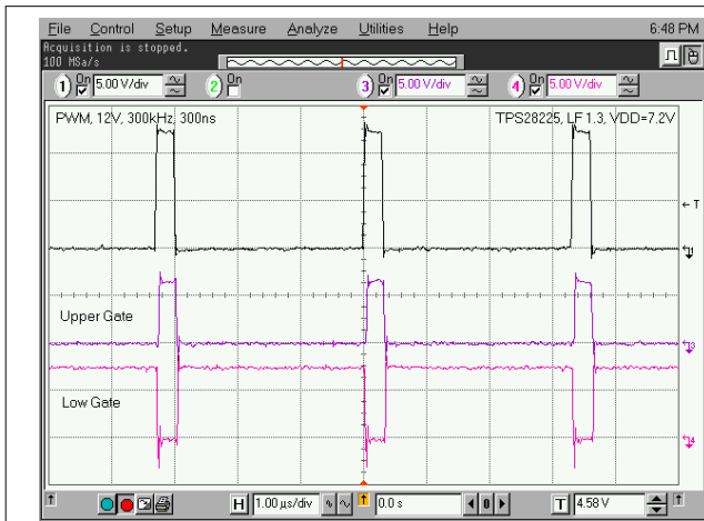
Figure 6-4. 12-V PWM Pulse at V_{DD} = 7.2\text{ V}
