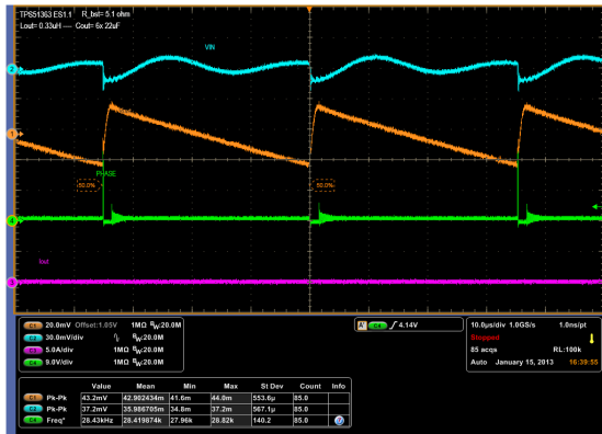
Figure 19. f = 800\text{kHz} , V_{IN} = 20\text{V} , I_{OUT} = 0.1\text{A}
