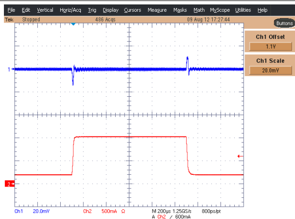
Figure 73. DCDCx Load Transient Response, 1.1 V_{OUT} , 200-1000-200 mA Load
