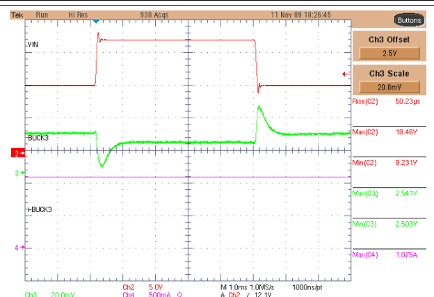
Figure 30. BUCK2 Transient Supply Response L_O = 4.7 \mu\text{H} , C_O = 22 \mu\text{F} , V_{OUT} = 2.5 \text{ V} , \Delta V_{IN} = 9 \text{ V to } 8 \text{ V}
