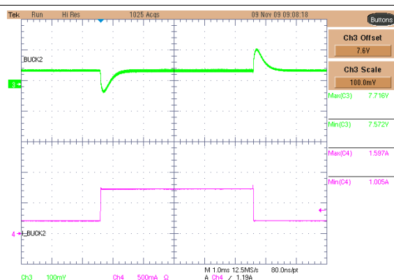
Figure 33. BUCK3 Transient Load Response L_O = 4.7\text{ }\mu\text{H} , C_O = 22\text{ }\mu\text{F} , V_{OUT} = 7.5\text{ V} , \Delta I = 1\text{ A to }1.5\text{ A}
