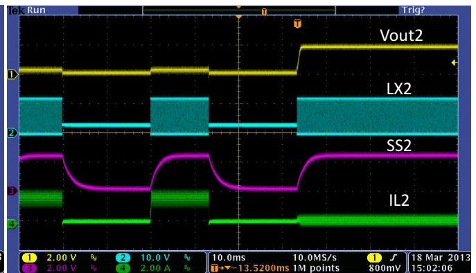
Figure 35. Hiccup Recover, Buck2=1.8V
