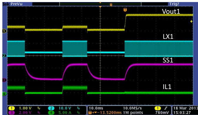
Figure 34. Hiccup Recover, Buck1=1.2V
