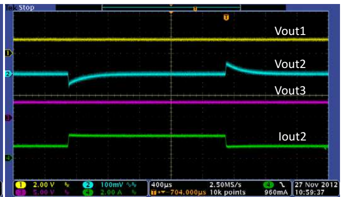
Figure 23. Transient Response Buck2@1.8V, 1-2A Step, C_o = 47\ \mu\text{F}
