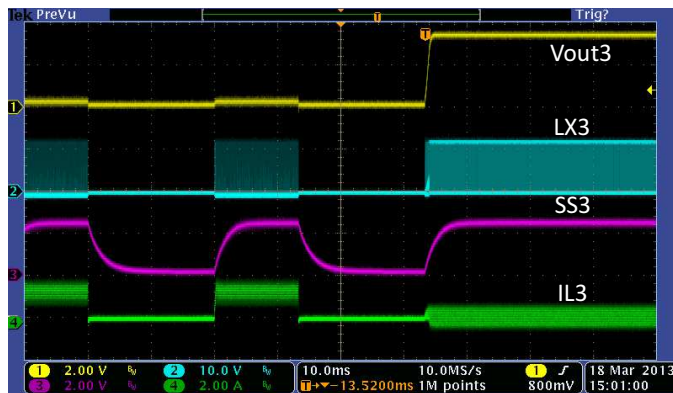
Figure 36. Hiccup Recover, Buck3=3.3V
