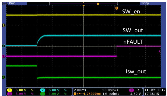
Figure 40. USB Switch Current Limit Recovery
