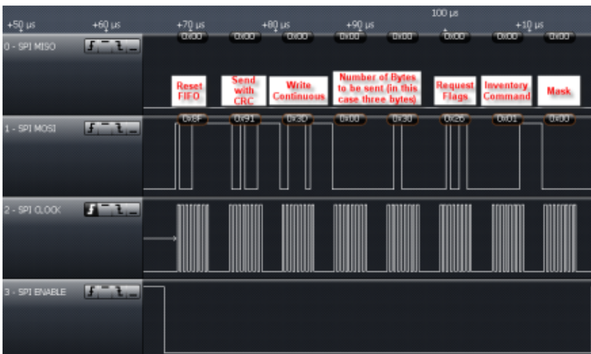
Figure 6-22. Inventory Command Sent From MCU to TRF7970A
