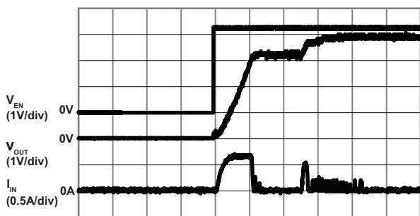
Soft Start (V OUT = 3.8V; V IN = 3.3V; I OUT = 0A)
