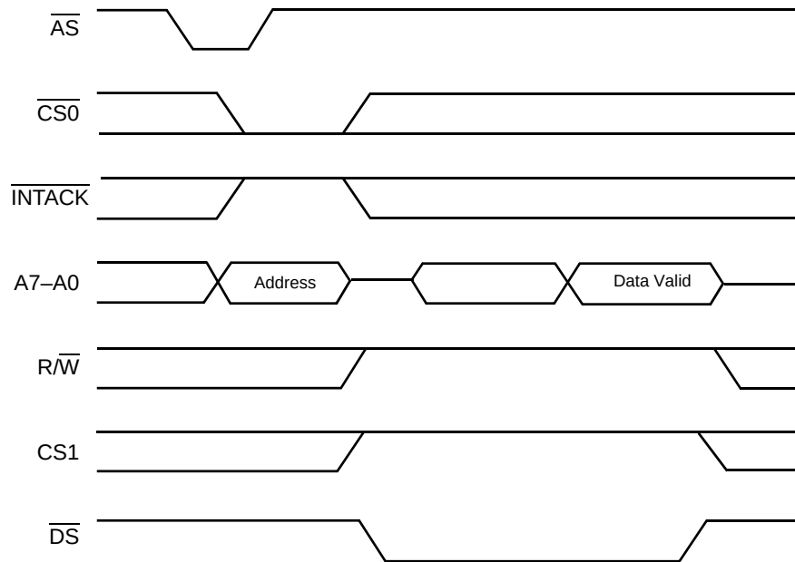
Figure 18. Z80230 Read Cycle Timing
