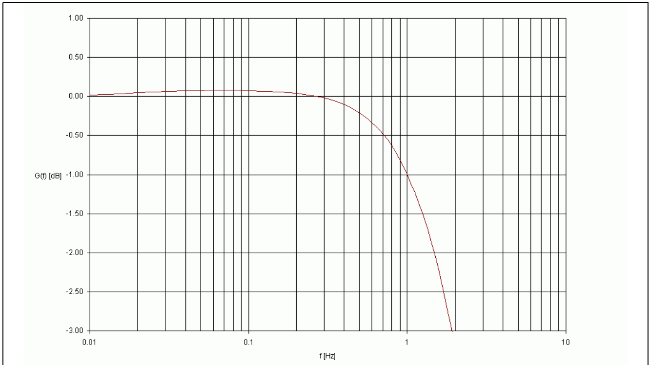
Figure 26 - Jitter Transfer Function - Detail
