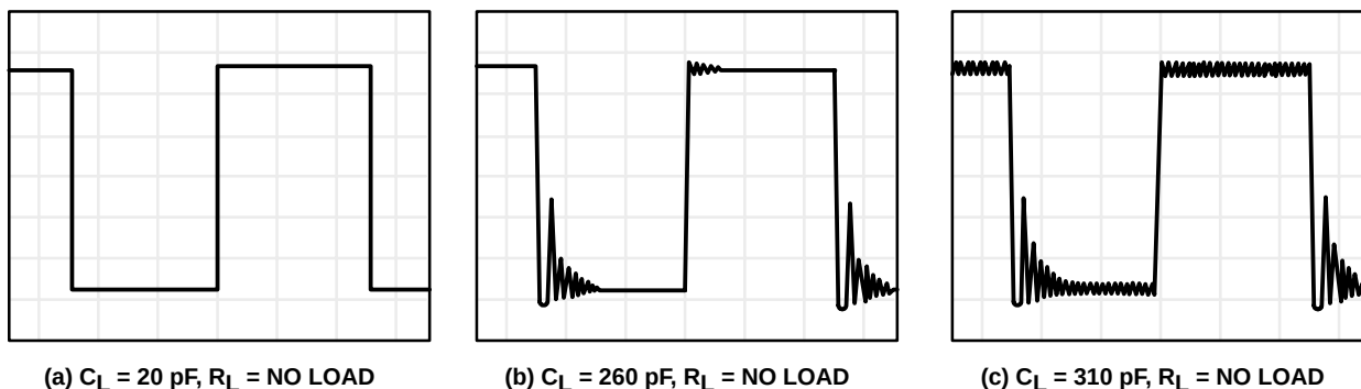
Figure 112. Effect of Capacitive Loads in Low-Bias Mode
