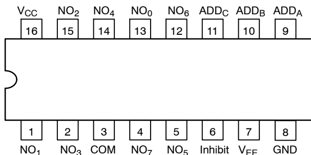
Figure 1. Pin Connection (Top View)
