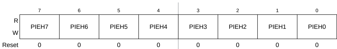
Figure 23-54. Port H Interrupt Enable Register (PIEH)
