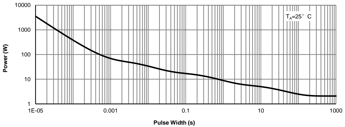
Figure 14: Single Pulse Power Rating Junction-to-Ambient (Note H)
