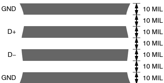
Figure 22. Arrangement of Signal Tracks
