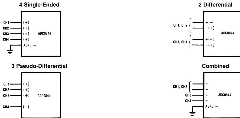
Figure 12. Analog Input Multiplexer Options
