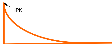
Figure 26. Input Charge Inrush Current
