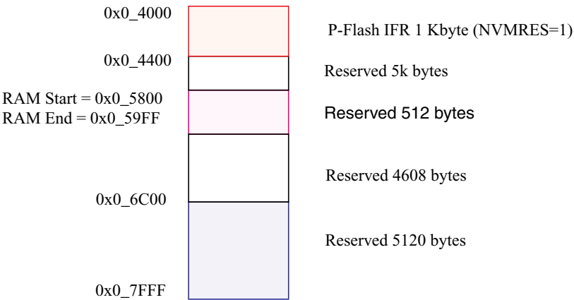
Figure 24-3. Memory Controller Resource Memory Map (NVMRES=1)
