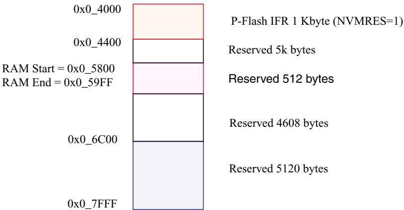
Figure 25-3. Memory Controller Resource Memory Map (NVMRES=1)
