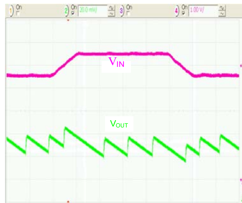
Figure 22. Line Transient Response in PFM Mode, 10\text{ }\mu\text{s/div} .
