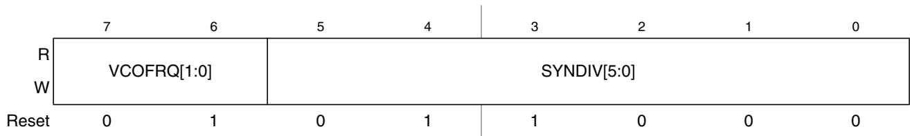
Figure 10-4. S12CPMU Synthesizer Register (CPMUSYNR)
