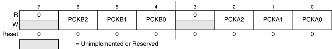
Figure 19-6. PWM Prescale Clock Select Register (PWMPRCLK)
