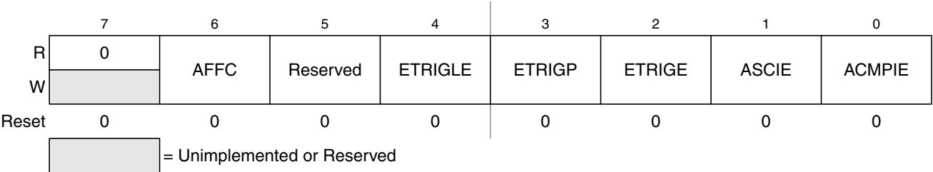
Figure 16-5. ATD Control Register 2 (ATDCTL2)
