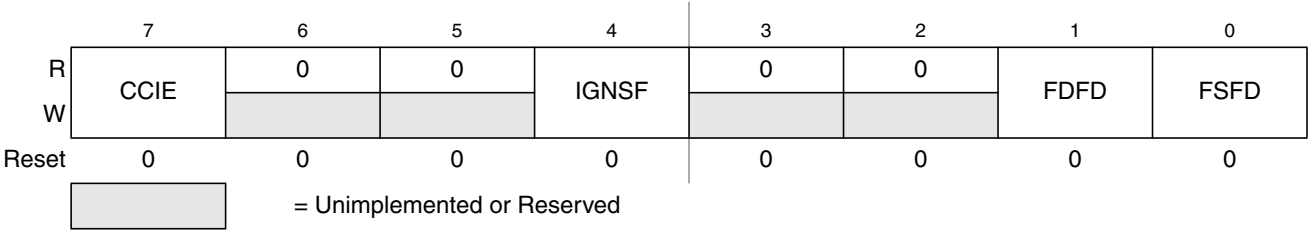
Figure 25-9. Flash Configuration Register (FCNFG)
