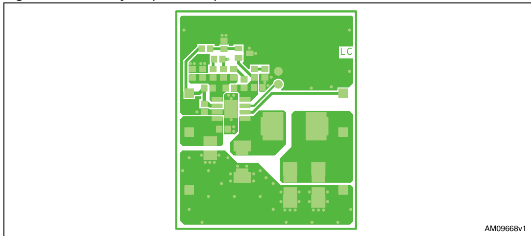
Figure 25. PCB layout (front side)
