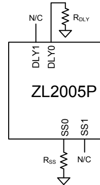
Figure 15. DLY and SS Pin Resistor Connections
