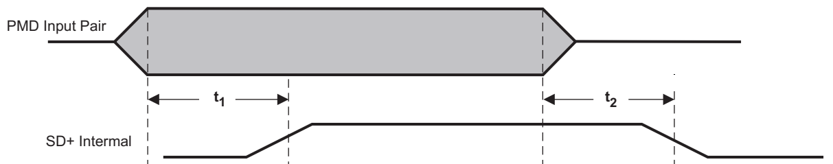
Figure 9-20. 100Base-TX Signal Detect Timing
