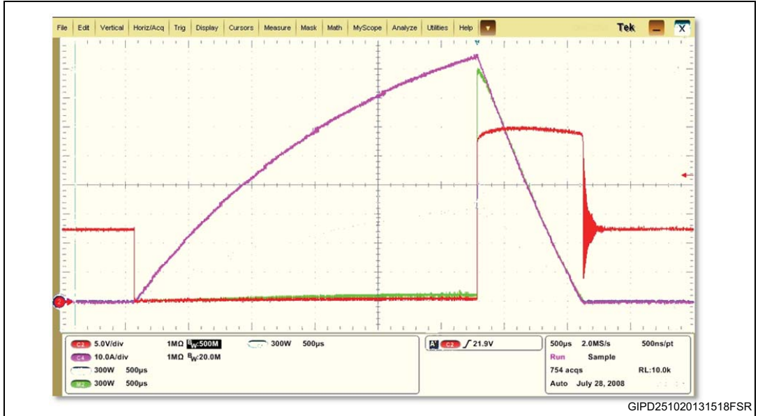
Figure 26. Unclamped inductive switching - experimental waveforms
