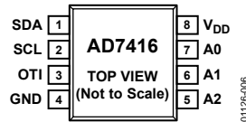
Figure 7. AD7416 Pin Configuration (SOIC/MSOP)
