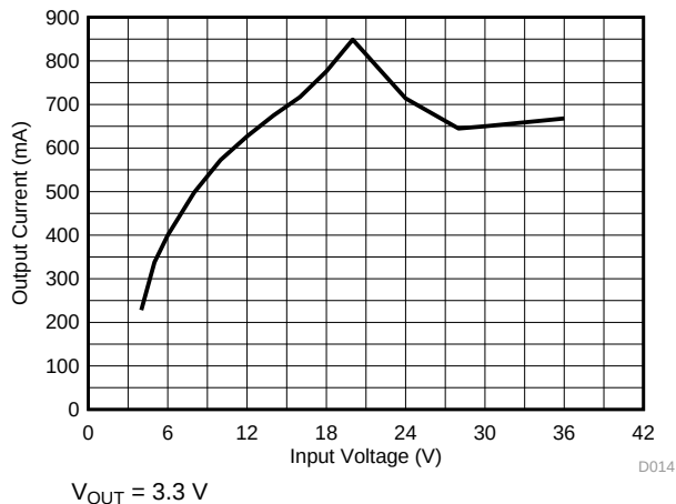
Figure 44. Load Current for PFM-to-PWM Transition
