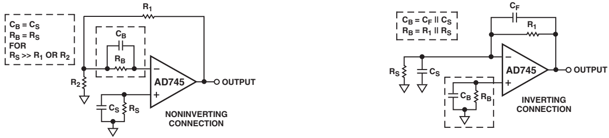
Figure 40. Optional External Components for Balancing Source Impedances
