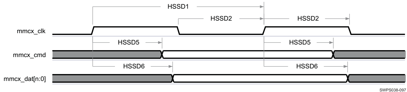
Figure 6-74. MMC2 and MMC3 Interfaces—High-Speed SDIO Mode—Data/Command Transmit (1)
