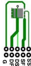
d. 120\text{ }^\circ\text{C}/\text{W} when mounted on a minimum pad of 2 oz copper
