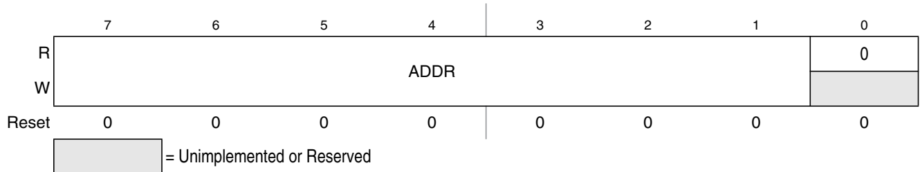
Figure 13-3. IIC Address Register (IIC1A)
