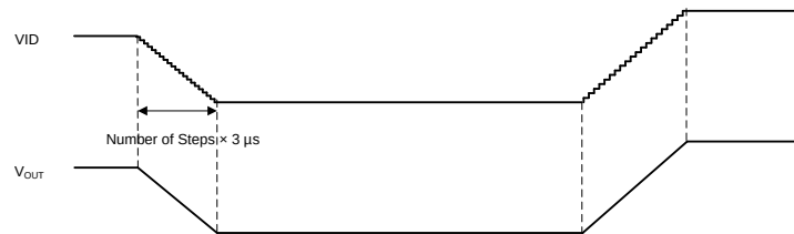
Figure 6-5. DVS Timing Diagram I
