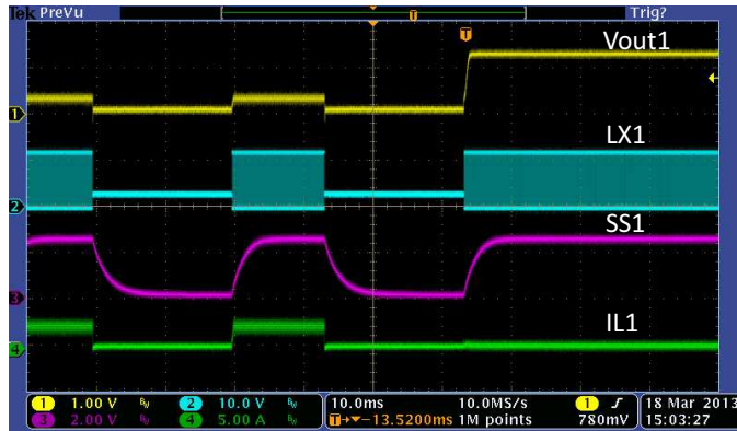
Figure 34. Hiccup Recover, Buck1=1.2V
