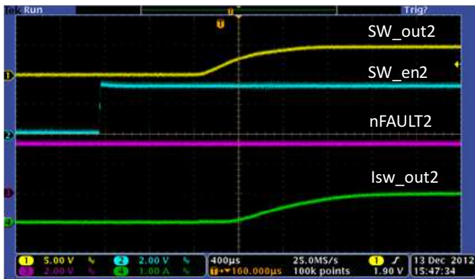
Figure 40. USB Switch2 Start-Up 1A Load
