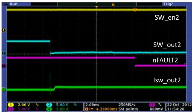
Figure 42. USB Switch2 Current Limit Operation
