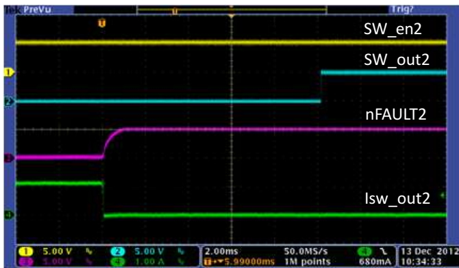
Figure 44. USB Switch2 Current Limit Recovery
