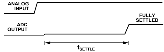
Figure 61. Step Input with Single Cycle Settling
