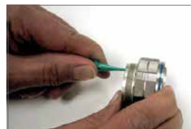
Plastic tool with contact in proper position.
