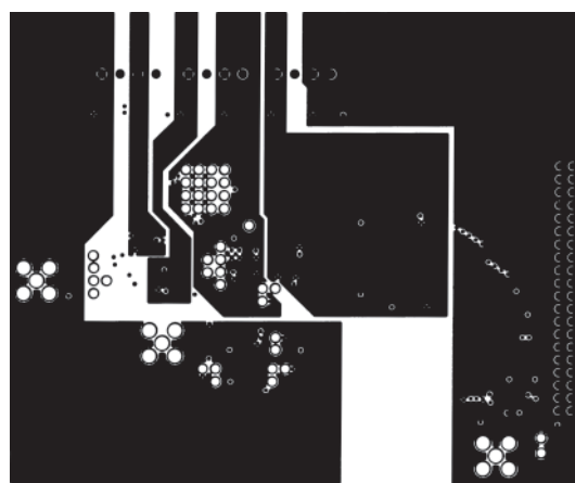
Figure 15. PCB Ground Layer—Layer TBD
