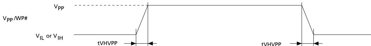
Figure 24: Accelerated Programming Timing Waveform
