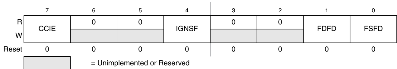
Figure 25-9. Flash Configuration Register (FCNFG)
