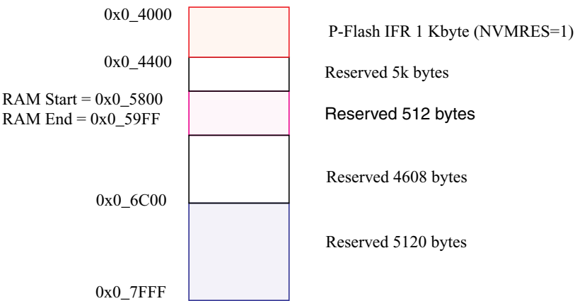
Figure 26-3. Memory Controller Resource Memory Map (NVMRES=1)
