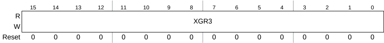
Figure 6-14. XGATE Register 3 (XGR3)
