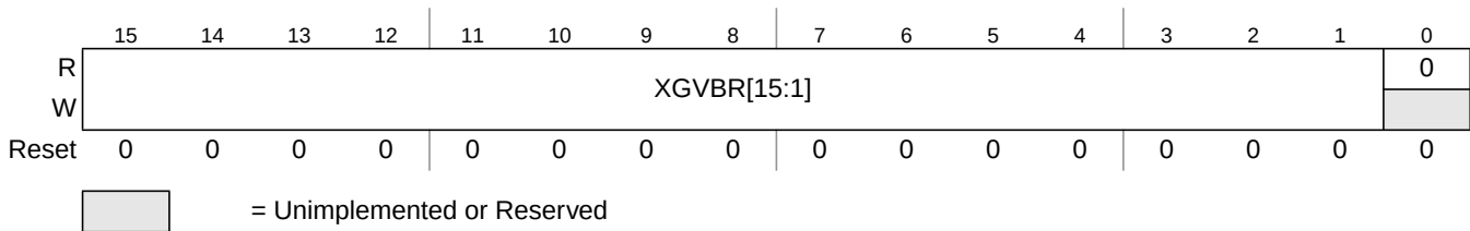
Figure 6-5. XGATE Vector Base Address Register (XGVBR)
