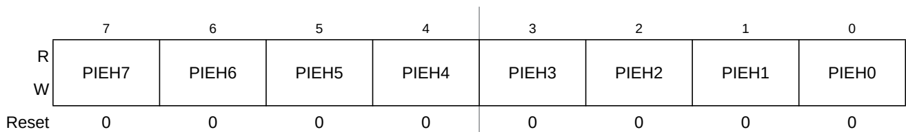
Figure 23-54. Port H Interrupt Enable Register (PIEH)
