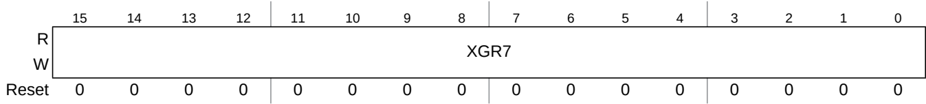
Figure 6-18. XGATE Register 7 (XGR7)
