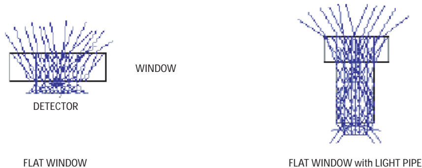
Figure 12. Recommended window design.
