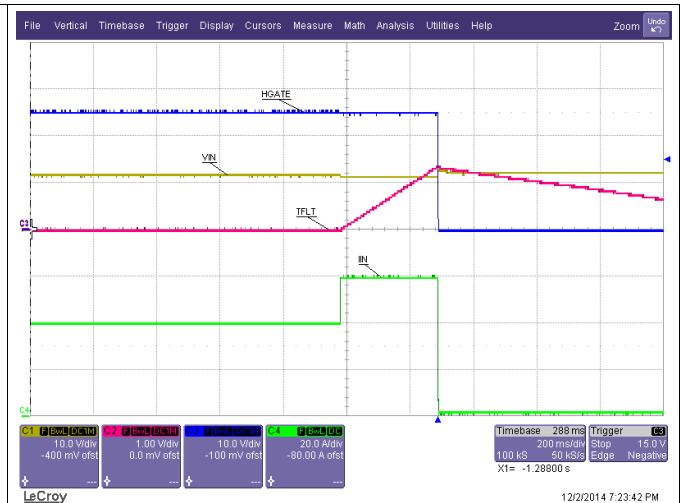
Figure 55. Load Step 40A to 60A
