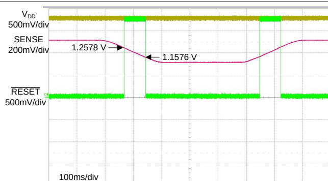
Figure 35. Window Comparator Thresholds Entering a Valid Window
