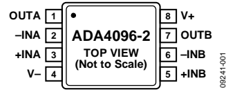
Figure 1. 8-Lead, MSOP (RM-8), ADA4096-2
