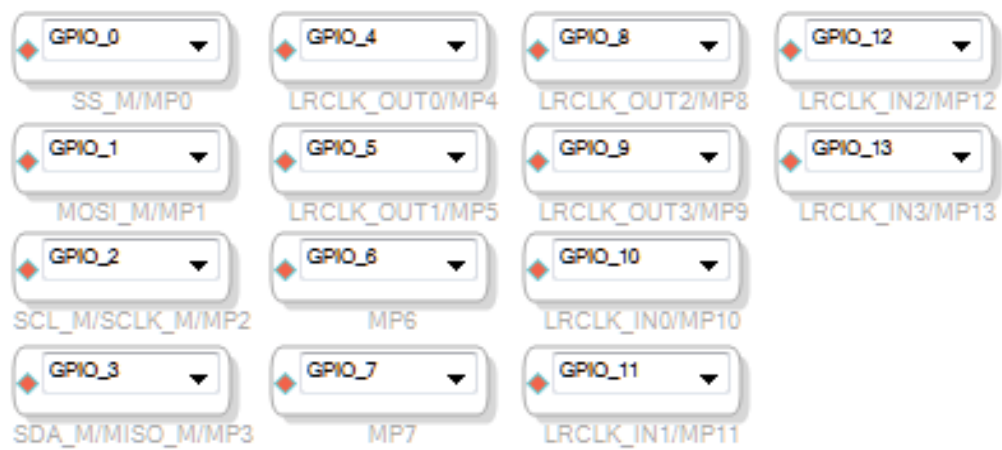
Figure 76. Complete Set of General-Purpose Outputs in SigmaStudio
