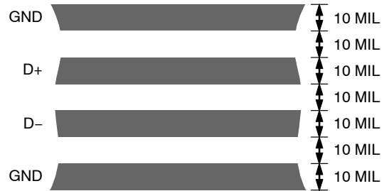
Figure 18. Arrangement of Signal Tracks
