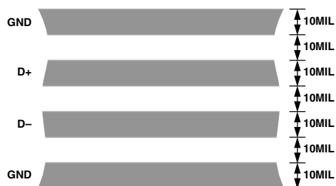
Figure 8. Arrangement of Signal Tracks
